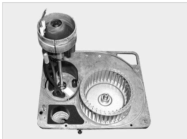
Abb. 67: Brenner in Serviceposition
