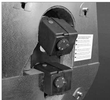
Installed electrical heating elements and flange insulation
