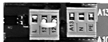
L/13/12 with jumper on 12 - 13
