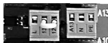
L/13/12 with jumper on 12 - 13
