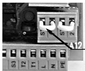
ST1/ST2 with jumper on ST - 2
