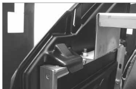
Hanging the side covers in to place
