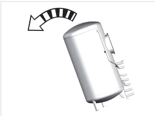
Fig.2: Tilting the storage tank
