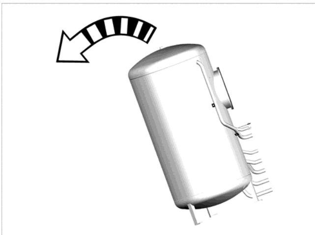
Fig.2: Tilting the storage tank
