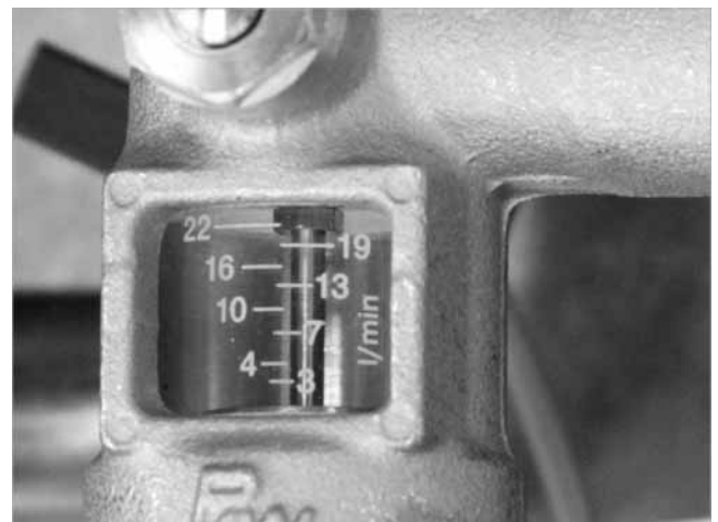
Fig. 18: Read the volume flow at the upper edge of the float
