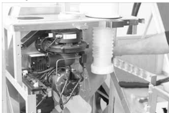
Fig. 13: Aligning the exhaust connection piece
