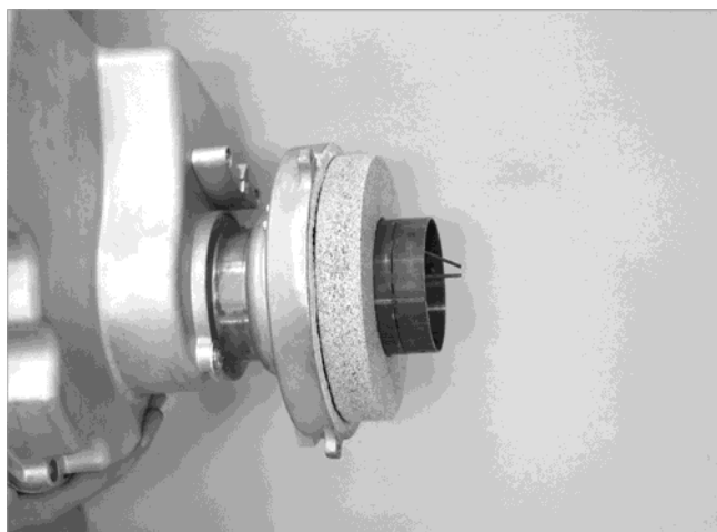
Fig. 5: Putting the firebrick in place
