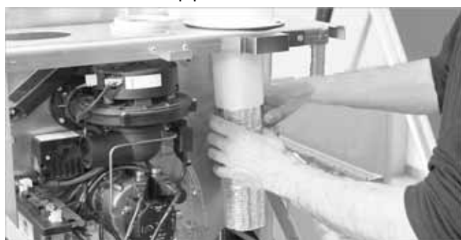
Fig. 11: Inserting the internal pipe silencer
