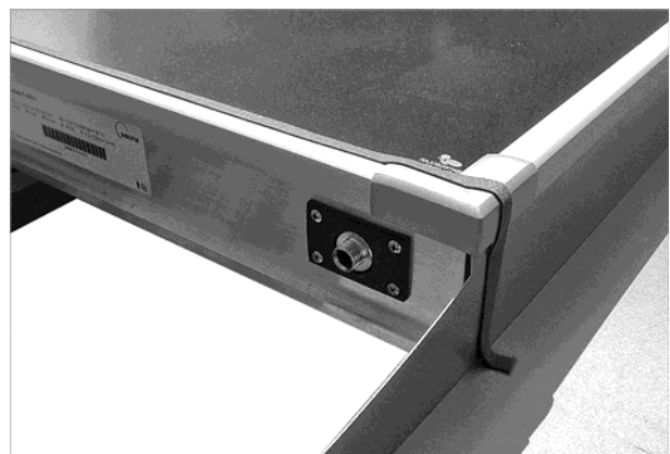
Fig. 78: Sticking the joint sealing strip on the upper edge along the entire width of the profile
