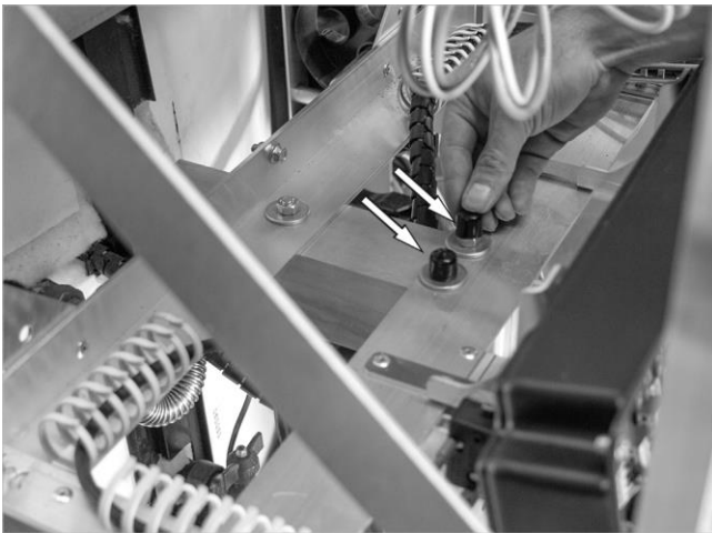
Fig. 10: Covering the screw heads on the console
