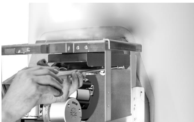
Fig. 14: Screwing the bellows seal bracket tightly
