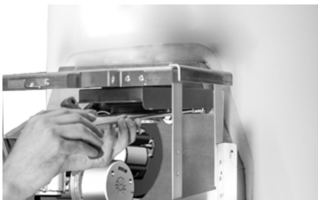
Fig. 14: Screwing the bellows seal bracket tightly
