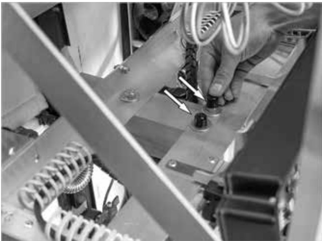
Fig. 10: Covering the screw heads on the console
