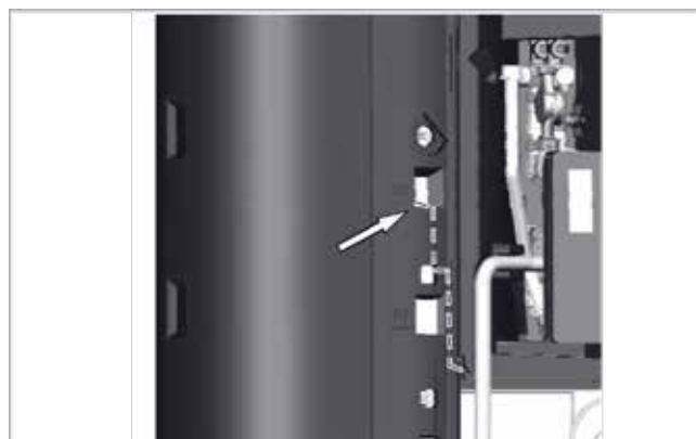
Abb. 23: Sensor S1 in Position S1-Eco montieren
