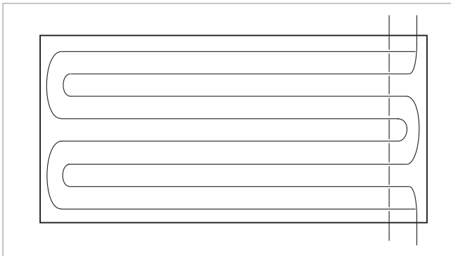
Fig. 6: Hydraulics of SolvisFera Integral (F-xx3-I-AR)
