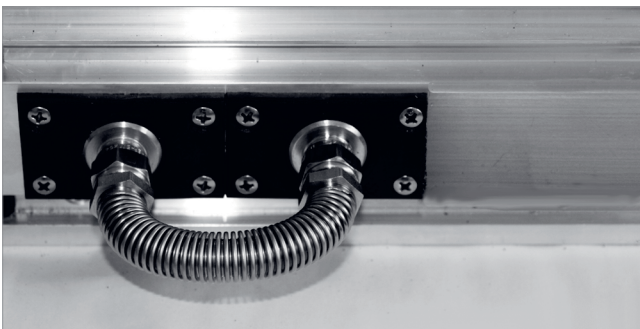
Fig. 50: Installed connection elbow
