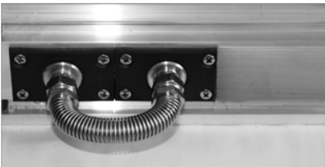
Fig. 50: Installed connection elbow
