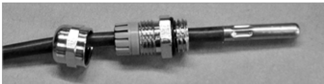
Fig. 70: Pushing the PG screw fitting onto the collector sensor
