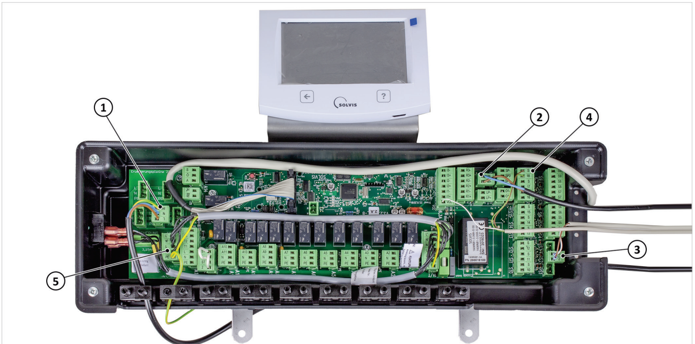
Fig. 6: SolvisControl 3 mains module
