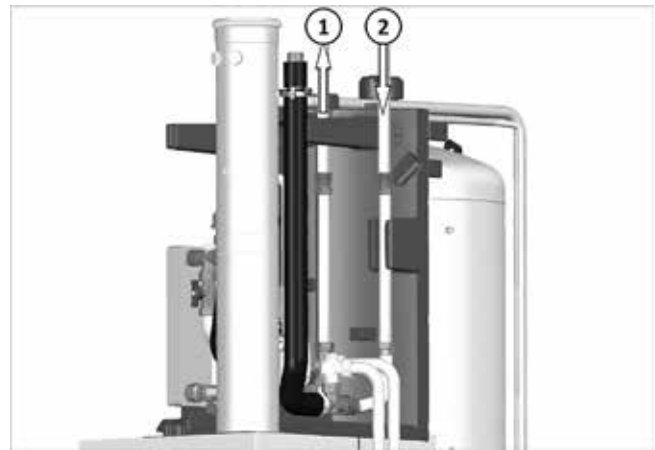
Fig. 39: H-VL/H-RL connection from above
