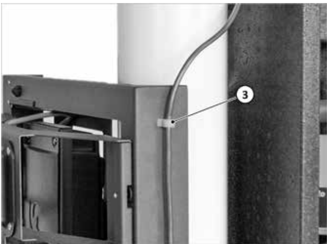
Fig. 83: Fastening the oil supply line to the frame
