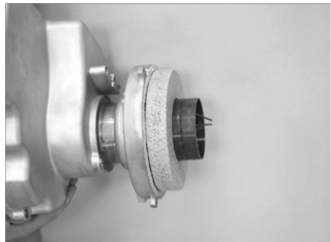
Fig. 68: Putting the door firebrick in place
