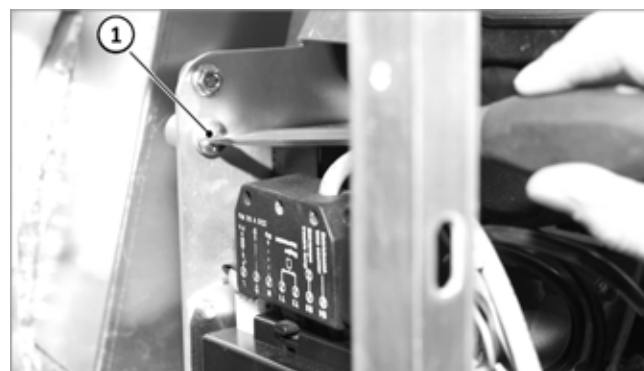
Fig. 144: Quick release screws on the burner insert
