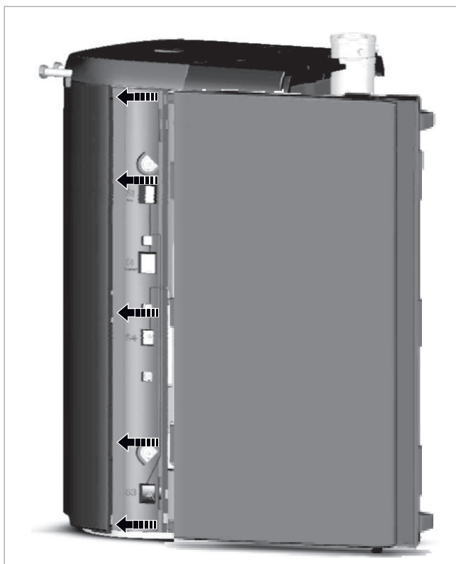
Fig. 134: Adding the side section
