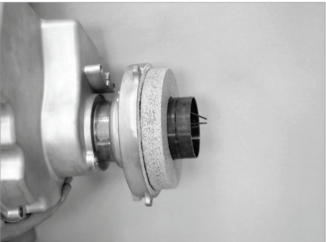
Fig. 68: Putting the door firebrick in place
