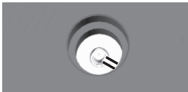
Fig. 81: Bleeder hose on the bleeder
