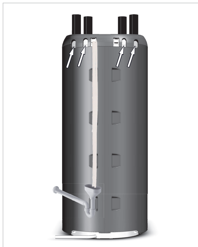
Fig. 72: Fleece plugs on the rear side
