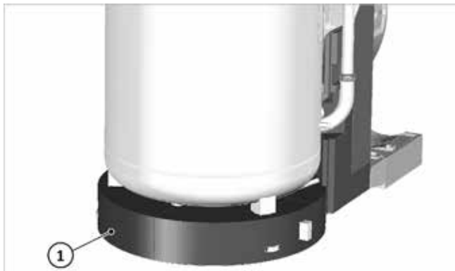
Fig. 12: Placing the floor disc under the storage tank
