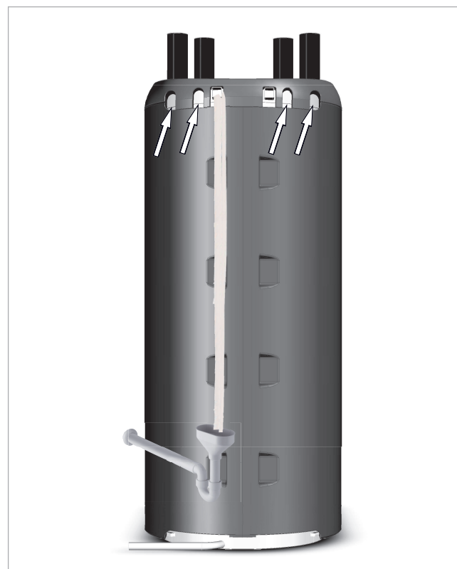
Fig. 72: Fleece plugs on the rear side
