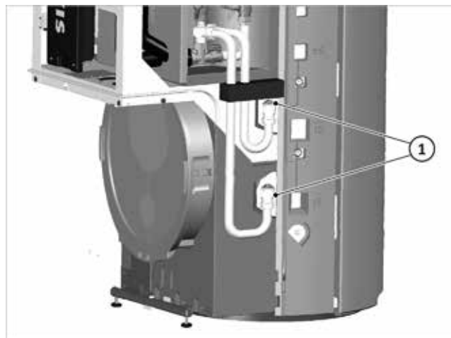
Fig. 30: Checking/retightening the heating circuit station connections
