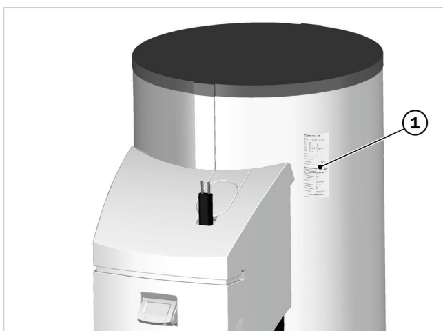
Fig.108: Nameplate (1) attached to the insulation
