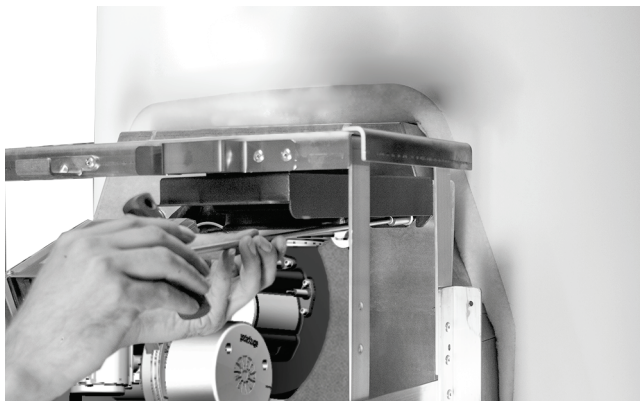
Fig. 34: Screwing the bellows seal bracket tightly
