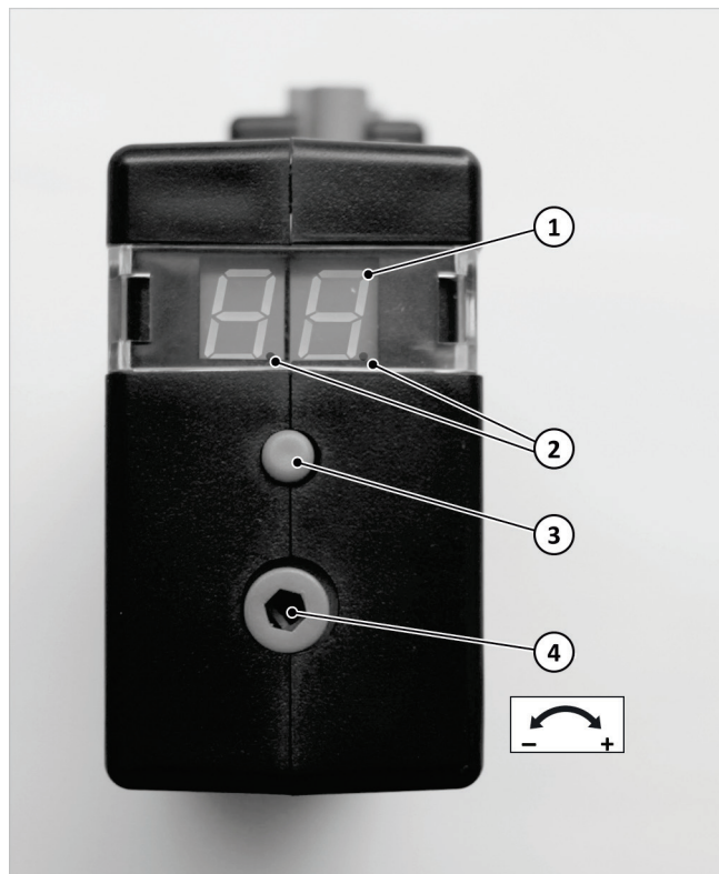
Fig. 121: Interface for automatic firing system CM 168
