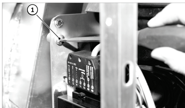
Fig. 113: Quick release screws on the burner insert
