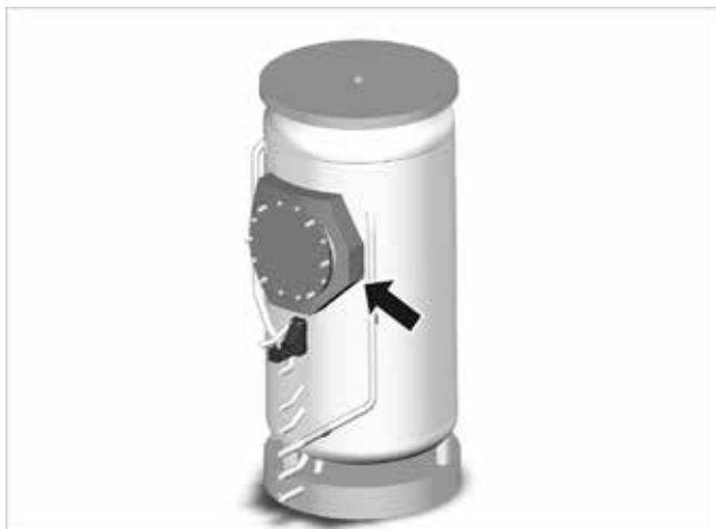
Fig.5: Fit the flange collar shell
