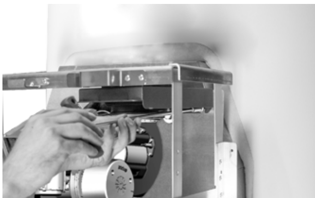
Fig. 34: Screwing the bellows seal bracket tightly
