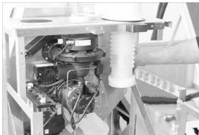
Fig.61: Aligning the exhaust connection piece
