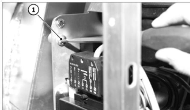
Fig. 113: Quick release screws on the burner insert
