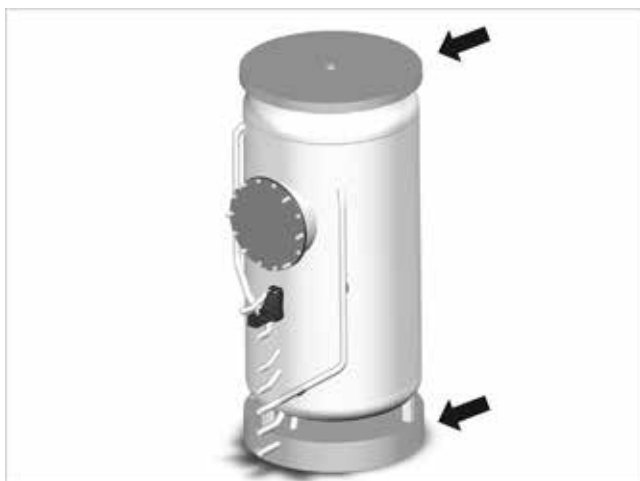
Fig.4: Position the floor and cover base plates
