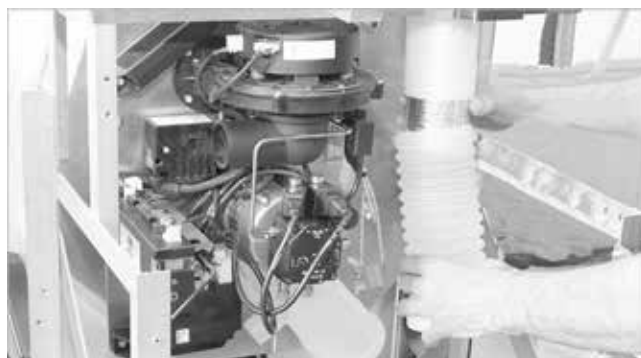
Fig.60: Connecting the exhaust connection piece
