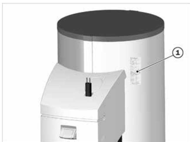
Fig.108: Nameplate (1) attached to the insulation
