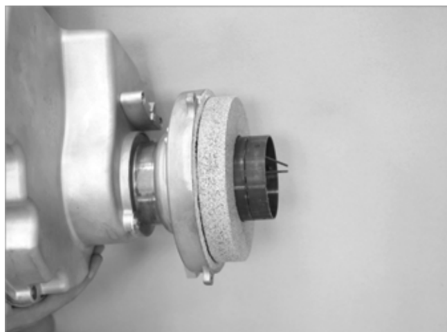
Fig. 53: Putting the firebrick in place
