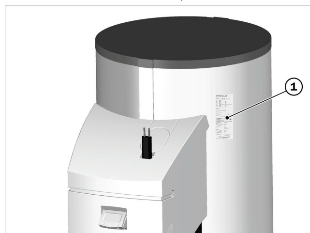
Fig.30: Nameplate (1) attached to the insulation
