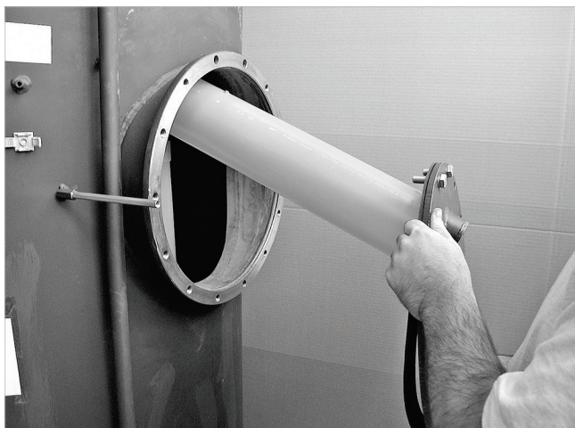
Fig. 3: Inserting the flange cover
