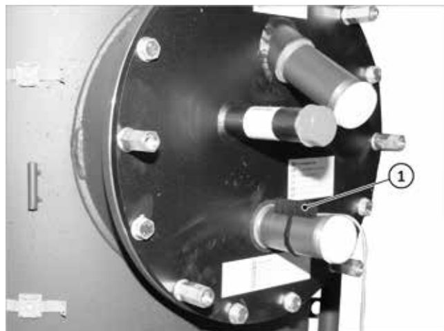
Fig. 4: Sensor S4 (1) fitted
