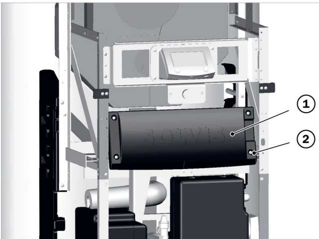
Fig. 19: Attach the cover of the mains circuit board
