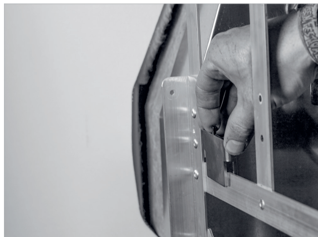
Fig. 116: Hanging the support hook
