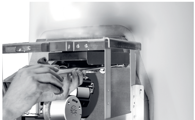
Fig. 38: Screwing the bellows seal bracket tightly
