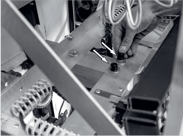
Fig. 34: Covering the screw heads on the console
