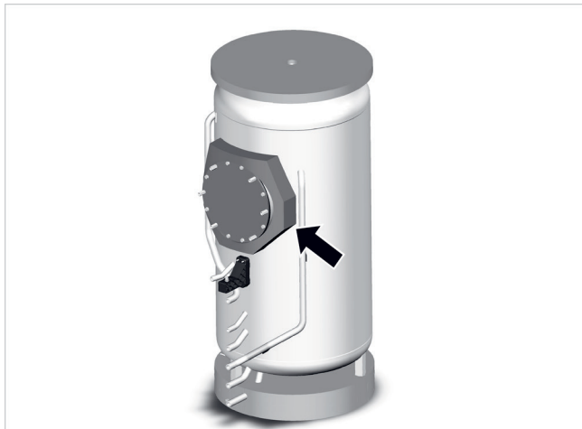
Fig.5: Fit the flange collar shell
