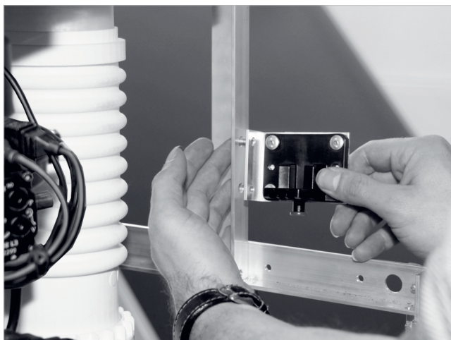
Fig. 67: Attaching the oil filter bracket
