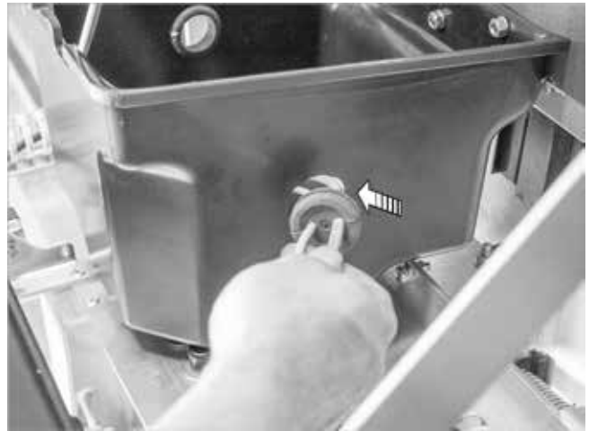
Fig. 36: Airtight lead-through for the burner cable
