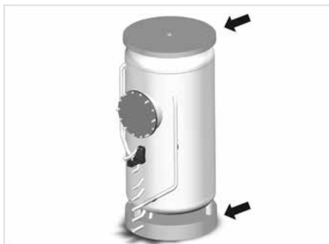
Fig.4: Position the floor and cover base plates
