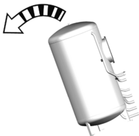
Fig.1: Tilting the storage tank
