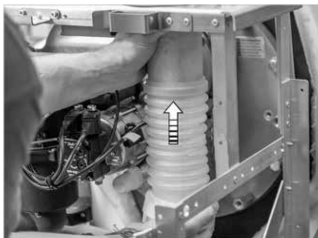
Fig. 63: Connecting the exhaust connection pipe section
