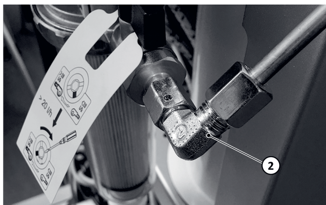
Fig. 78: Connecting the oil supply line to the filter
