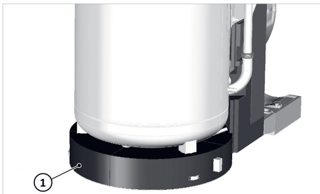
Fig. 13: Placing the floor disk under the storage tank
