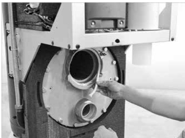
Fig. 46: Inserting the burner sealing cable
