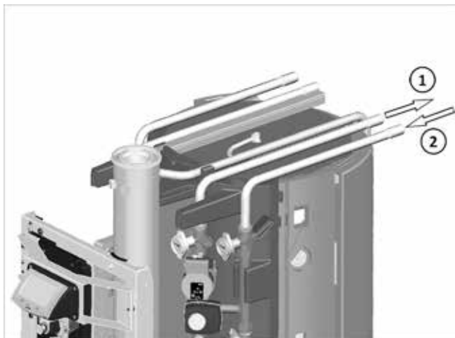
Fig. 34: H-VL/H-RL connection from the rear
