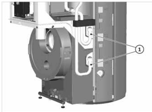
Fig. 31: Checking/retightening the heating circuit station connections
