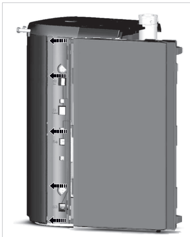
Fig. 129: Adding the side section
