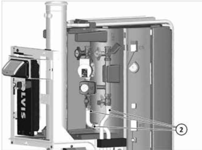
Fig. 5: Removing the pipe sections (2)
