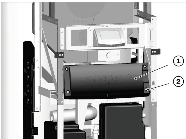
Fig. 21: Attach the cover of the mains circuit board
