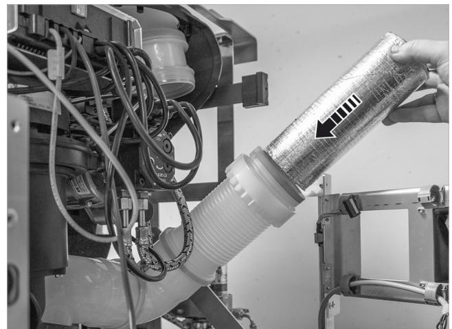
Fig. 79: Insert the long silencer at the bottom
