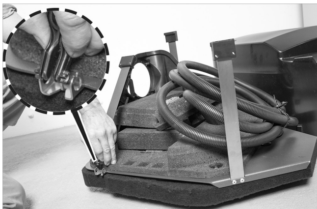
Fig. 12: Disassemble the locking rail
