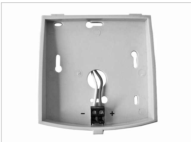
Fig. 115: Connect the room controller
