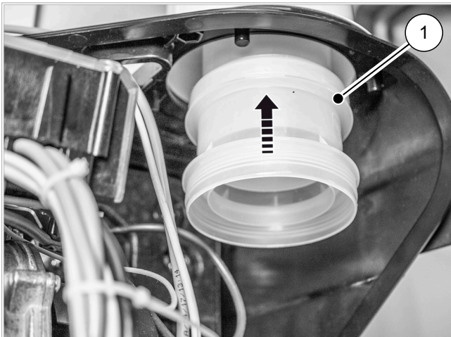
Fig. 76: Attach the flue pipe coupling to the flue pipe connection piece.
