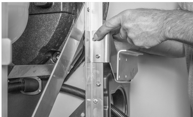
Fig. 63: Attaching the oil filter bracket
