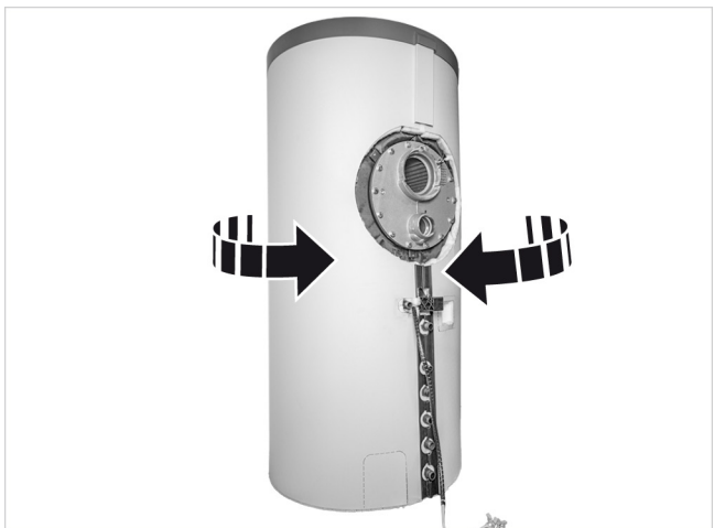
Fig. 6: Insulating the storage tank
