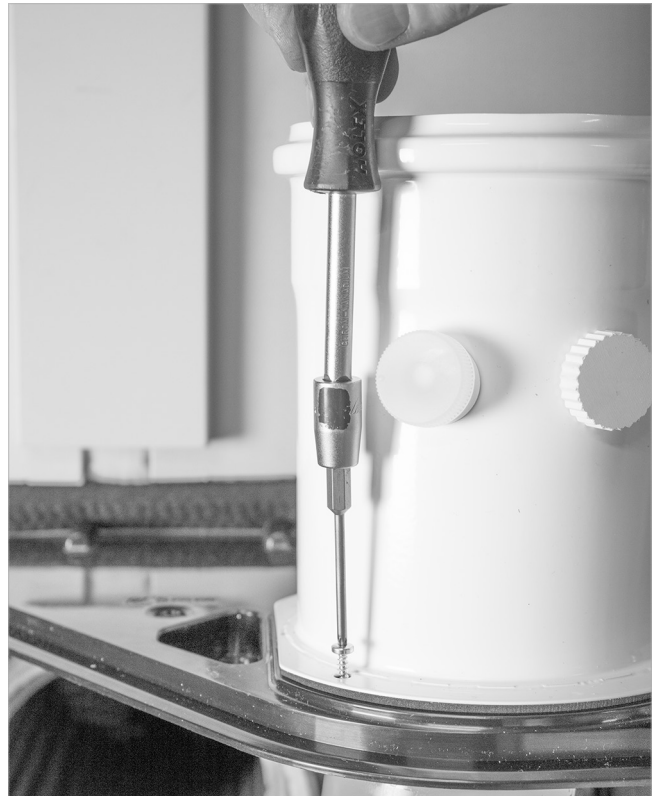
Fig. 37: Fit the exhaust connection piece
