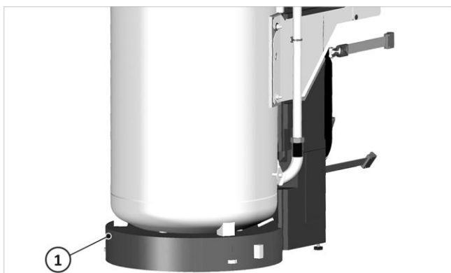
Fig. 15: Placing the floor disk under the storage tank
