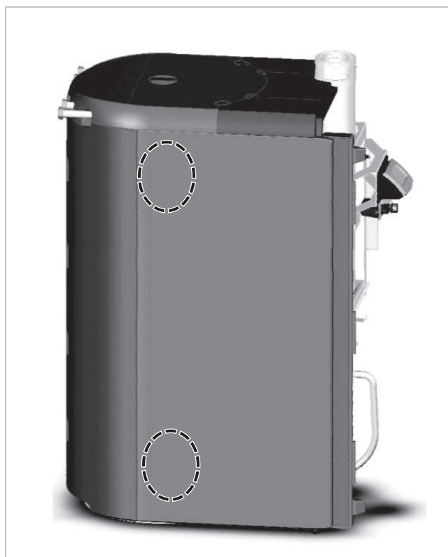
Fig. 136: Pushing in the side panel
