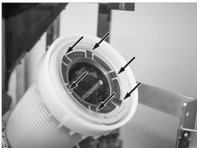
Fig. 83: Lock the star ring
