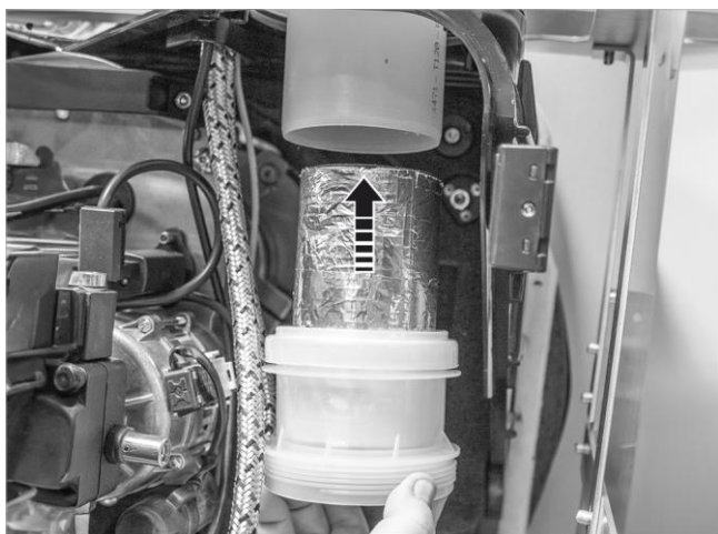
Fig. 81: Insert the short silencer at the top
