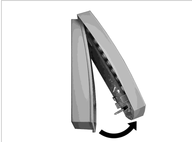
Fig. 110: Opening the housing
