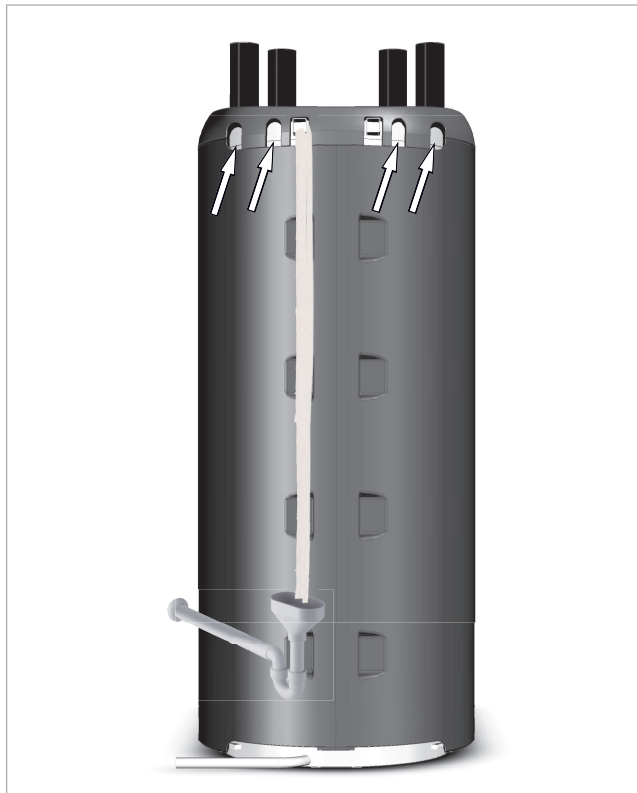
Fig. 132: Fleece plugs on the rear side
