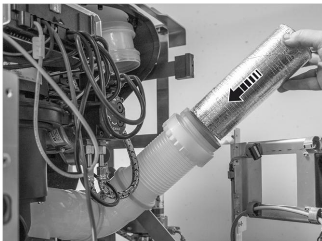
Fig. 82: Insert the long silencer at the bottom
