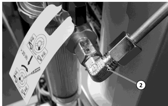
Fig. 73: Connecting the oil supply line to the filter
