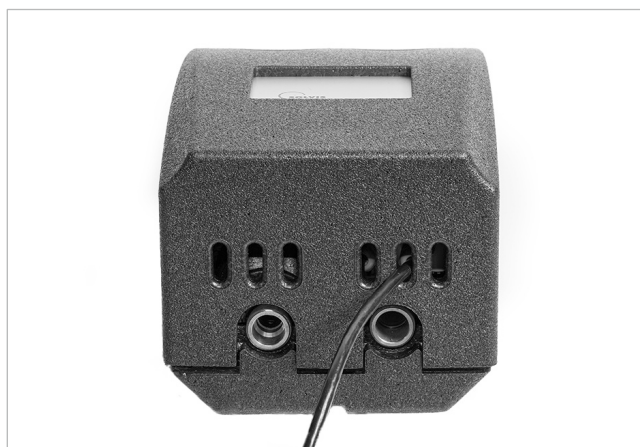
Fig. 9: Modbus cable routed through ventilation slot
