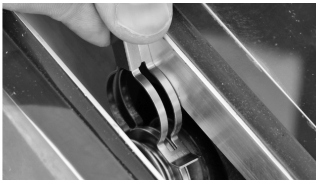
Fig. 23: Attaching the locking clip
