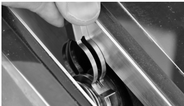
Fig. 46: Attaching the locking clip
